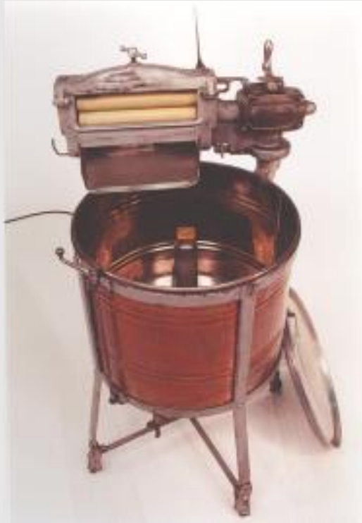
Figure 9.23 A pre-WWII washing machine produced by Beatty Brothers. Note the wringer – or mangle – in which children’s fingers are going to get squished.
