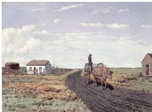
Figure 8.17 Red River carts were amphibious craft consisting of a flatbed attached to two large, convex spoked wheels. No metal was used in their construction and the wheels could be removed and strapped to the bottom so that the vehicle became a raft. They were invariably pulled by oxen. (Painting by William Hind, ca. 1862)
